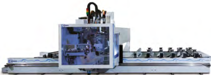
Machine bed of Nanodur® concrete – HOMAG Sorb Tech®
